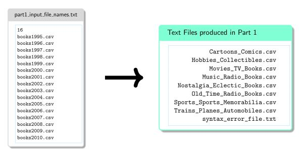
Preparing the input files for Part 2, Part 1 will output nine files, eight CSV-formatted text files and a regular text file, whose names are listed in the above box at right.
